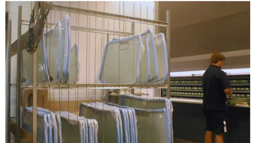
The HI280 shelving system is manufactured from pre-galvanized steel on a fully automated production line resulting in a product with high and consistent quality. The design is based on the principle of the minimum number of components possible. The lack of need for reinforcing cross bracing has resulted in a design that provides the max storage for its depth.
