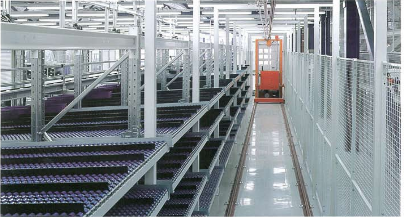
An automated feeder makes for simple loading of the SELECTAFLO system.
